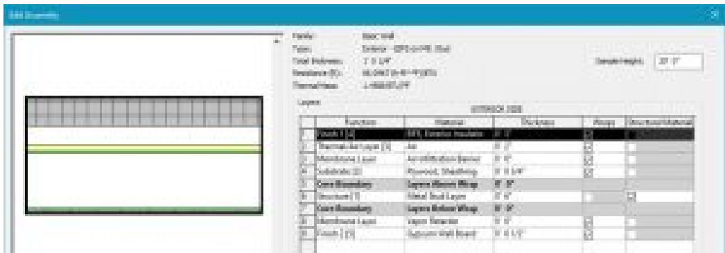
Figure 2.10 Basic Wall Exterior – EIFS on Mtl. Stud
