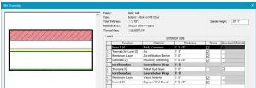
Figure 2.7 Basic Wall Exterior – Brick on Mtl. Stud
