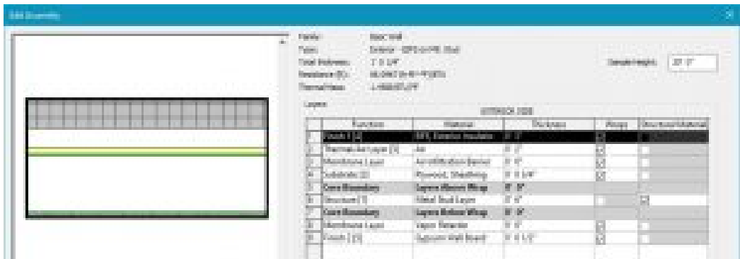
Figure 2.10 Basic Wall Exterior – EIFS on Mtl. Stud
