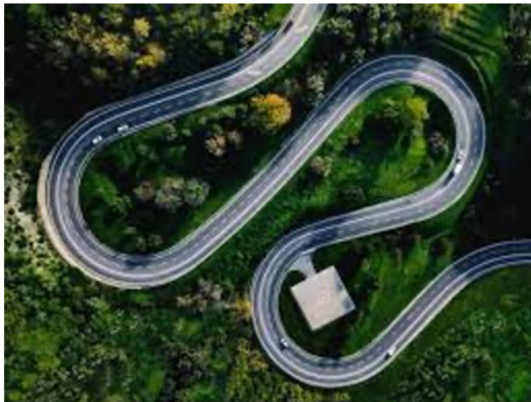
Figure 1: Horizontal profile (top view) of a road with significant horizontal curvature.
